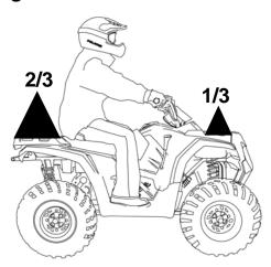
Your ATV has been designed to carry or tow a certain amount of load. Always read and understand the load distribution warning labels on the vehicle, and never exceed the weight capacities outlined in the specifications section of the owner's manual and on the safety decals.
